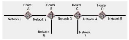
Router B uses RIP and has poison reverse enabled. Which cost metric does Router B advertise on Network 2 regarding Network 7?
