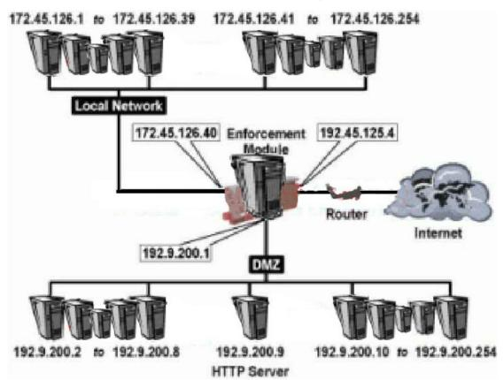
You want hide all localnet and DMZ hosts behind the Enforcemenet Module, except for the HTTP Server (192.9.200.9). The HTTP Server will be providing public services, and must be accessible from the Internet.
