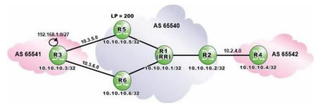
Router R1 is a route reflector with clients R2, R5 and R6. Prefixes advertised by router R5 have a local preference of 200. Router R3 advertises the prefix 192.168.1.0/27 to routers R5 and R6. Assuming that none of the routers in AS 65540 is configured with "advertise-external", what is the expected output of "show router bgp routes" on router R5?
