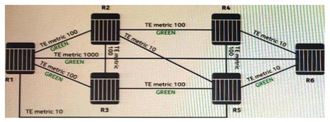
An LSP is being configured to start at R1and end at R6 using local CSPF. The LSP has the following constraints. Include admin-group GREEN, use the TE metric and hop-limit 3.
