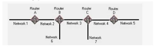
Router C uses RIP and has split horizon enabled. Which cost metric does Router C advertise on Netwok 3 regarding Network 6?
