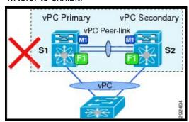
Customer has a pair of Cisco Nexus7010s switches and connected to a single Cisco Nexus5548 switch via vPC. Customer has a combination of M1 and F1 I/O Modules in Cisco Nexus7010s.
