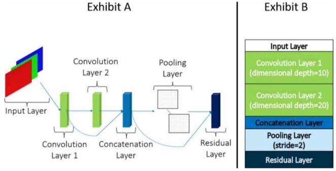
Exhibit A details the structure of a convolutional model Exhibit B provides details o( each layer in the model The blue arrowed lines represent connections between layers.
