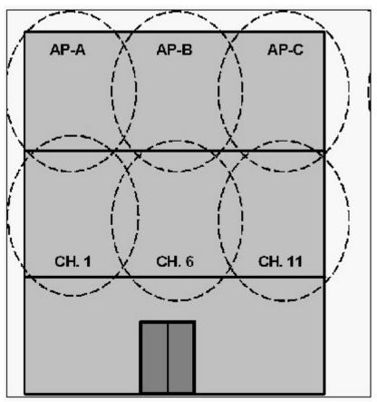
A.AP-A: channel 1, AP-B: channel 6 and AP-C: channel 11 B.AP-A: channel 7, AP-B: channel 8 and AP-C: channel 9 C.AP-A: channel 11, AP-B: channel 1 and AP-C: channel 6 D.AP-A: channel 2, AP-B: channel 3 and AP-C: channel 4 E.AP-A: channel 6, AP-B: channel 11 and AP-C: channel 1
