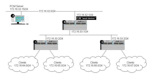
You have installed PCM+ and all of its plug-in applications on this network. You have not performed any additional configuration. How many subnets will be displayed in the navigation tree when you log in to PCM+ for the first time?
