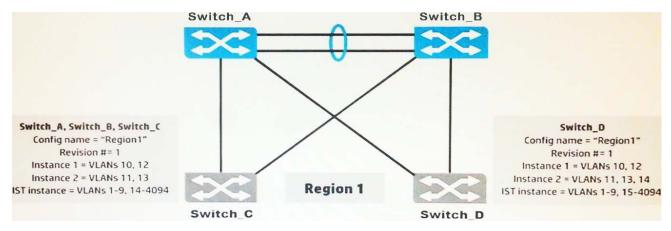
Originally, all four switches had the same region configuration. VLAN 14 was added to Switch\_D and then mapped to instance 2.
