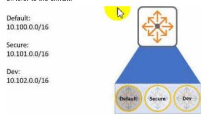
Aruba CX 6300 switch has routes in three different VRFs as per the example above. The user needs to leak routes between VRF Secure and VRF Dev. and also between VRF default and VRF Dev. The customer Is not able to establish routing between directly connected networks 10.100.50.0/24 and 10.102.26.0/24.
