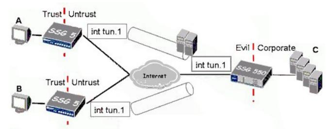
In the exhibit, the hub and spoke VPN uses route-based VPNs and has intra-zone blocking enabled on the Evil zone.
