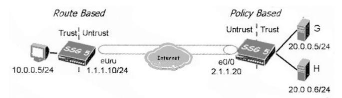
In the exhibit, the route-based VPN on the SSG 5 needs to configured to allow access only from your PC to Server G. The SSG 550 is configured with a policy-based VPN from Server G to your PC's host address.
