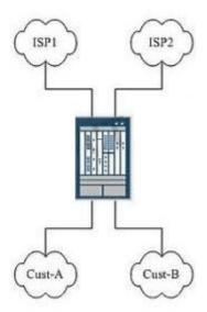
In the exhibit, Customer A and Customer B connect to the same SRX Series device. ISP1 and ISP2 are also directly connected to the SRX device. Customer A's traffic must use ISP1, and Customer B's traffic must use ISP2.
