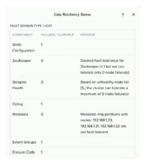
An administrator notices that the Data Resiliency Statue of some components has been reduced to 0. making it impossible to support a node failure in the cluster.
