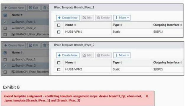
Exhibit A shows two IPsec templates to define Branch\_IPsec\_1 and Branch\_IPsec\_2. Each template defines a VPN tunnel.
