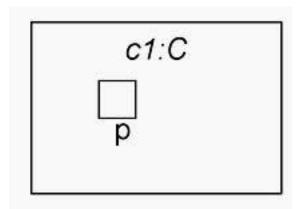
A. p is a port on a part of composite C, which is not shown.
