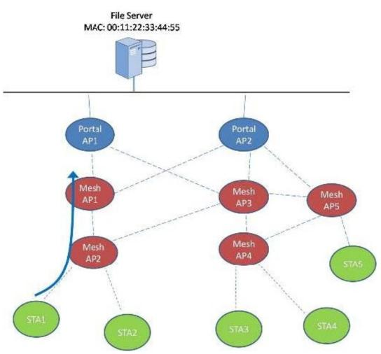
STA1 sent a data frame to Mesh AP2 destined for a local file server on the same subnet with MAC address 00:11:22:33:44:55. Mesh AP2's mesh forwarding algorithm determined that the frame should be forwarded through Mesh AP1.
